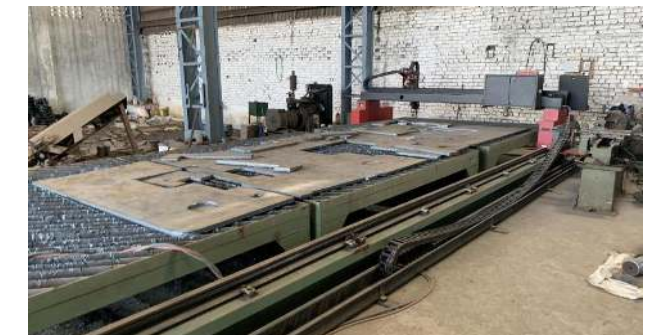
CNC Oxy-Fuel Cutting 3000mm x 12000mm
